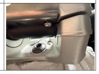
Using a T25 in a small driver, tighten the two bolts securing the bracket to the handlebar clamp casting. Press up from the bottom of the T25 bit to achieve ratcheting action while tightening the bolts.
